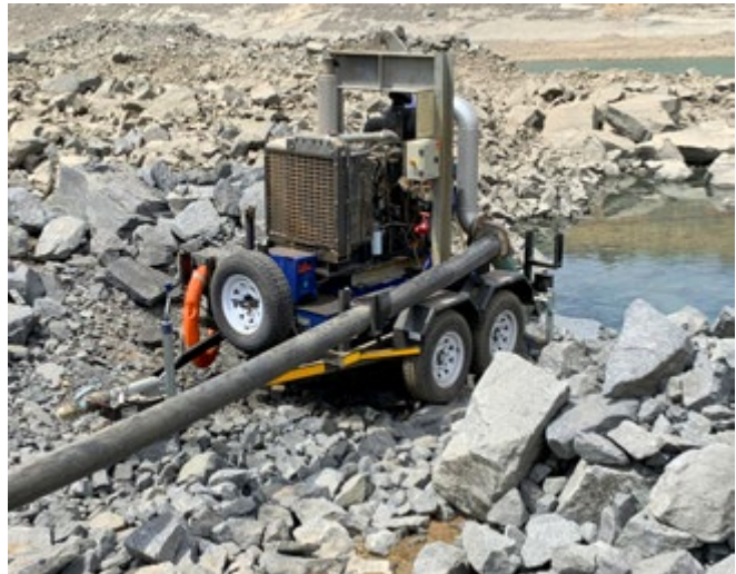
The Sykes CP units weigh 1,5 tons on a road trailer
